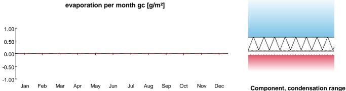
Condensation Risk Analysis calculations according to BS EN ISO 13788 are used as a guide in predicting interstitial condensation. This methodology uses some simplifications of the dynamic processes involved and subsequently does have some limitations. For further information the user is advised to follow the prescriptive guidance in BS 5250:2021 Management of moisture in buildings – Code of practice & BRE Information Paper:IP2/O5 (Feb. 2005) 'Modelling and controlling interstitial condensation
